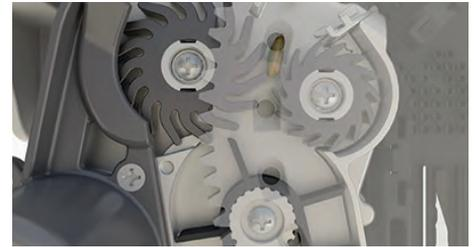
Feeder wheels grab the seed off the disk and place it onto the belt for delivery to the trench while maintaining superior singulation.
