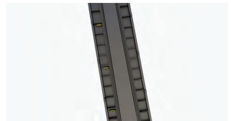
The belt controls the seed down the tube eliminating seed bounce and row unit ride issues.
