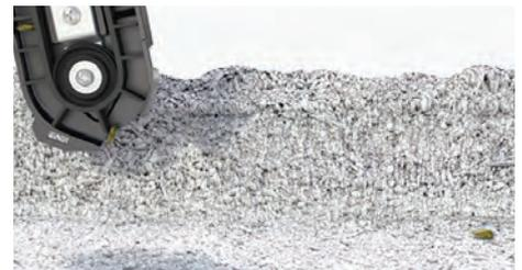
The belt matches the speed of the planter and drops the seed exactly where it needs to be as SpeedTube eliminates seed roll and bounce.
